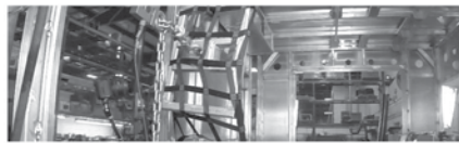
Safety Net pull tested to 3,000 lbs.
