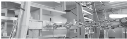
Cabinetry pull tested to 25X its weight, 9,000-11,000 lbs.
