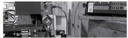
Cardiac Monitor pull tested to 10x Monitor + Tray weight, 550 lbs.
